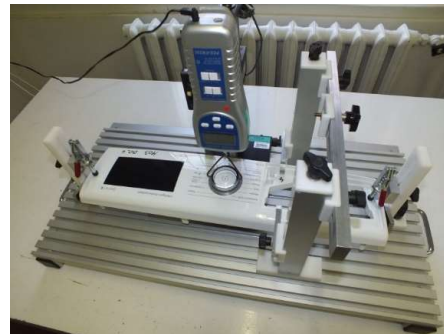
Actuation test bench for control panels (dryer)
