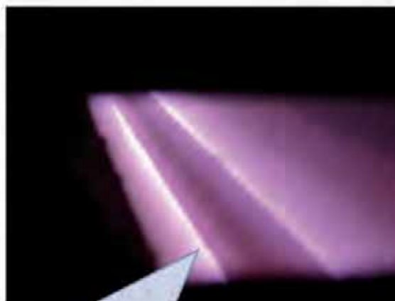
Linear microwave excited plasma source, wafers over- or underpass an array of up to 12 plasma sources for coating
